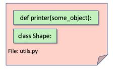
Thus, the printer() function and the class Shape are defined in the utils module. They can be referenced via the name of the utils module.
