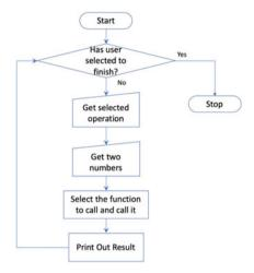
Based on this flowchart we can put in place the skeleton of the logic for the calculator's processing cycle.
