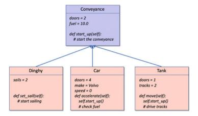
As an example, consider the class hierarchy illustrated above. A generic root class has been defined. This class defines a Conveyance which has doors, fuel (both with default values) and a method, start\_up(), that starts the engine of the conveyance. Three subclasses of Conveyance have also been defined: Dinghy, Car and Tank. Two of these subclasses are appropriate, but one should probably not inherit from Conveyance. We shall consider each in turn to determine their suitability.
