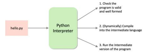
The way in which the Python interpreter processes a Python program is broken down into several steps. The steps shown here are illustrative (and simplified) but the general idea is correct.
